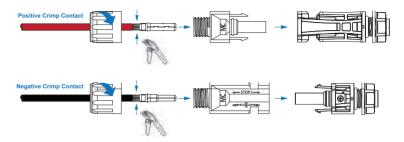
Note: Please use PV connector crimper to pinch the point of the arrow. You'll hear click sound when the connector assembly is correct.
