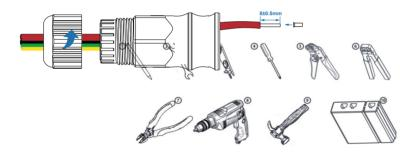
Note: The wiring terminals should be wrapped with insulation tape, otherwise it will cause a short circuit and damage the inverter.
