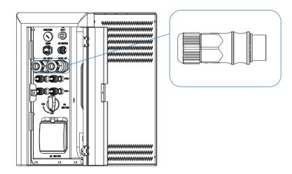
Note: After the wiring harness is locked, it should be pulled to prevent the locking from being unstable.
